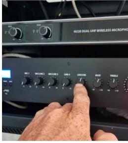
With volume slightly up on your device you can adjust the amplifier volume by slowly increasing the input volume using knob labelled “line/usb”
