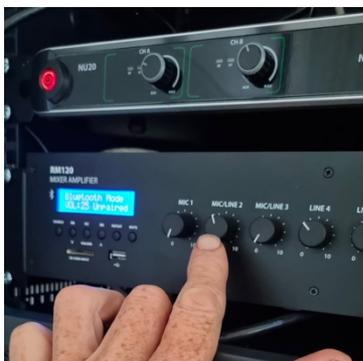
With the Large master volume set to around 3 or 4 slowly turn up the volume of the microphone input.
